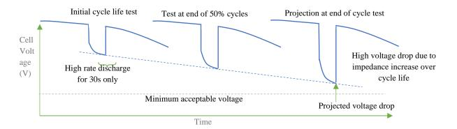
**Note:** Manufacturer should define the minimum acceptable voltage level. No "specific" value of the magnitude of the "high current" pulse is recommended for this test. The "manufacturer specified" 30 sec peak discharge current value shall be used for the test.
